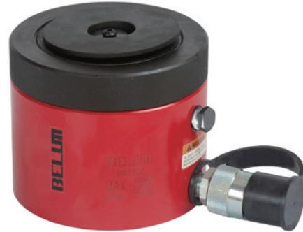
The BMLL-series is a design that features a threaded piston rod and lock ring. When the lock ring is screwed down and engaged with the cylinder body, the load can be held mechanically for extended periods. These cylinders are ideally suited to bridge construction and maintenance and jacking applications requiring safe extended load holding. All BMLL-Series cylinders feature a hard chrome bore for
