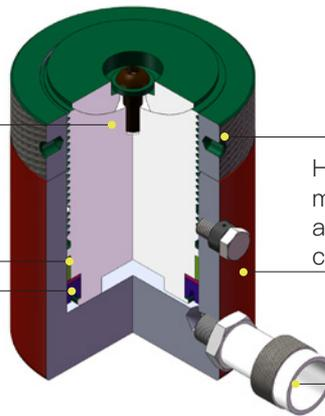
Mechanical locking nut design, long time load, more safe
